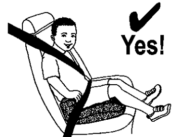
A booster helps seat belt fit properly. This is a backless booster.
